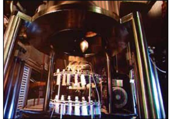
*GE - Aviation found that the VF-20 Induction Heating Vacuum Furnace provided accurate, consistent heating.*
