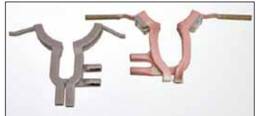
With GH microfusion technology, identical coils can be produced from the same 3D manufacturing mold. This increases repeatability and consistency when multiple induction systems are running the same process, and significantly reduces maintenance and calibration time when coils need to be changed out.
